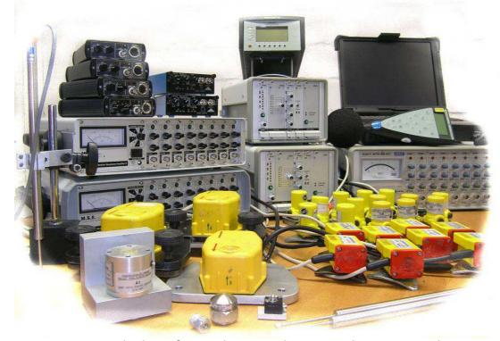
Measurements are the basis for nearly every vibration analysis. We attach great importance to the accuracy of our measuring instruments and the adequate state of all equipment. We are bound to a strict quality assurance system. All instruments are calibrated once a year. For that purpose we keep our own shaker with a gauged sensor system.
